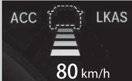
A vehicle icon with dotted-line contour appears on the driver information interface
