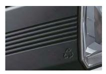
Front grille parts made of "recycled bumper material"
